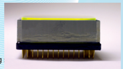
YAG:Ce - FOP - CCD System
