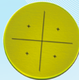
YAG:Ce Screen with Cross
