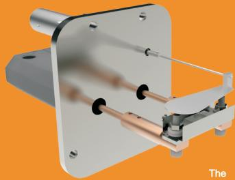
Thermal evaporation sources are generally used for basic thin film deposition processes. The evaporant material is placed in a conductive boat or alternatively a crucible held in a resistive coil. The boat or coil is heated by passing a high electrical current through it. As the temperature of the boat rises, the material in the boat begins to evaporate. The temperature, and hence the evaporation rate of the material, is controlled by the amount of applied current.
